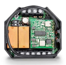
Receiving module for activating automatic doors and window drives with 24 V DC
